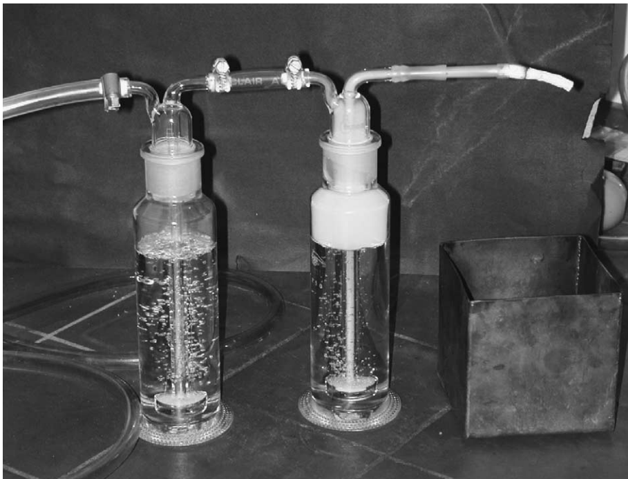
Fig. 4. Assembly for the collection of \Delta^9 -THC in smoking experiments. The smoke and the gases are sucked first through the right bottle and subsequently through the second left bottle.
